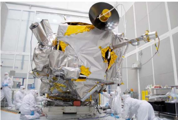
Photo Left: With the X-axis horizontal, we rotated to various positions for the blanket work. Here the team guides all of the cabling during a rotation.
