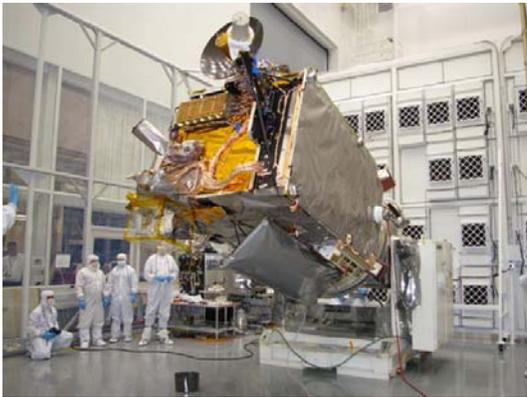
blanketing work, and we are now putting on the final touches for mass properties measurement, followed by mechanical environments.
