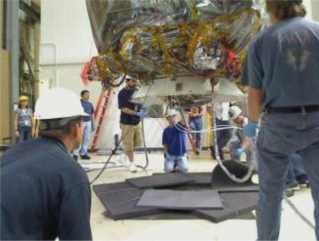
*The mechanical team prepares for the final shock test. During the test, an electrically actuated pin puller released the band mechanism, dropping the separation system on the foam pads. The flight separation system is painted white so that it doesn't get too hot in the sun while it travels with LCROSS to the Moon.*
