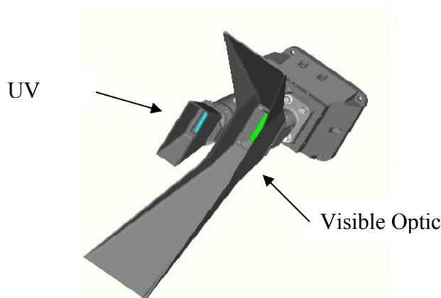
**Figure 7b LROC Wide Angle Component, 14.5 cm by 9.2 cm by 7.6 cm**
