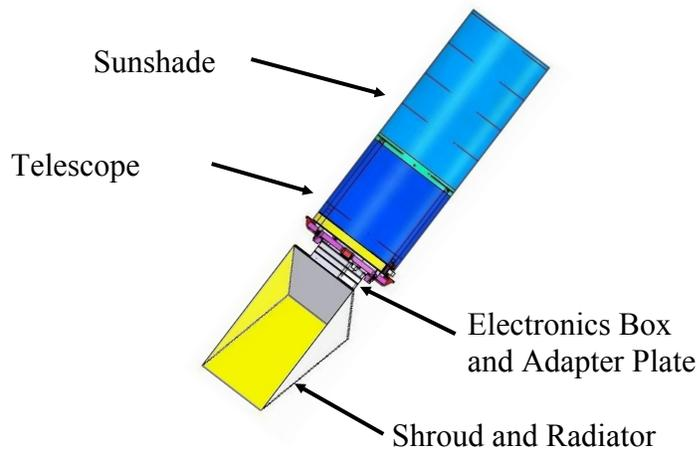
**Fig. 7a LROC Narrow Angle Component, 70 cm length by 24 cm diameter**
