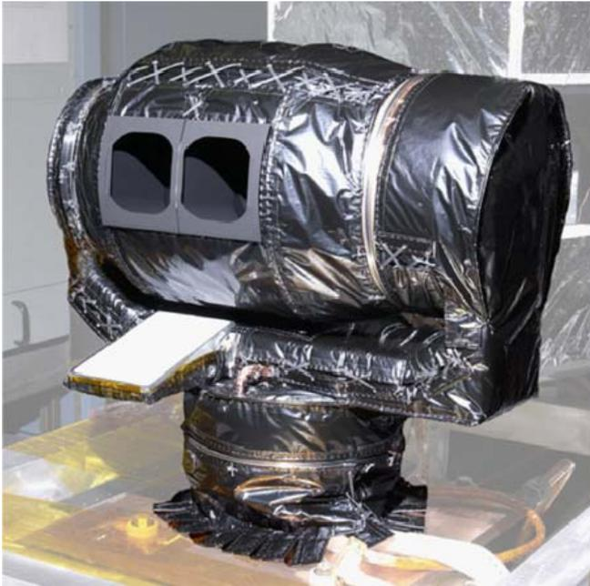
**Fig. 2** The MRO MCS Flight Model during thermal vacuum testing at JPL
