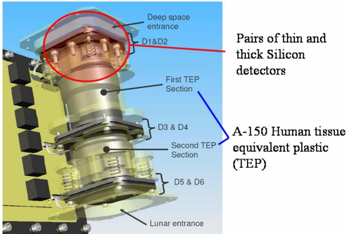
**Fig. 1. CRaTER Measurement Concept**
