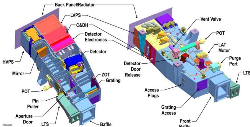
**Fig. 3** LAMP design as seen from above (left) and below (right).
