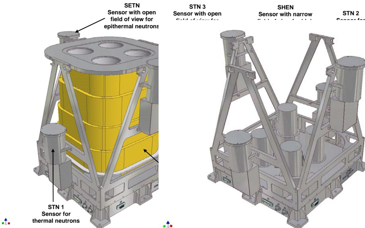
**Fig. 4 LEND Design Concept with four collimated sensors of epithermal neutrons CSETN 1-4, one sensor with narrow FOV for high energy neutrons SHEN and four sensors of thermal STN 1-3 and epithermal SETN neutrons with open fields of view. Left view is LEND with the collimator and right view is LEND without the collimator.**
