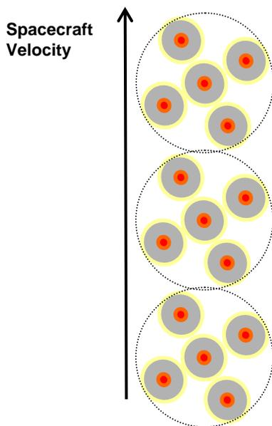
**Fig. 5. Pulse Detection Time-of-Flight Altimeter 5-spot Pattern Red represents the laser spots on the ground while the grey circles represent the receiver FOV.**
