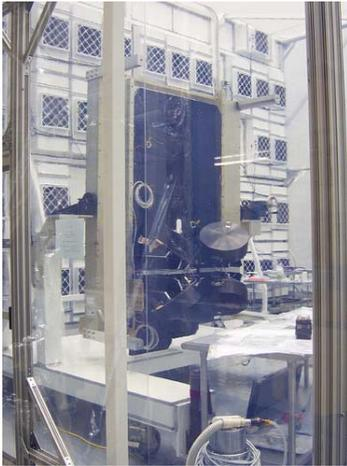
The reactions wheels, to the left, that will keep LRO stable in orbit have been integrated into one of the panels of the spacecraft bus.
