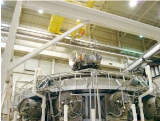
Here is the Orbiter being lifted out of the thermal vacuum chamber.
