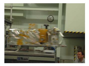
Instrument Module Sine-Burst Test
