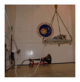
Instrument Module Acoustic Test
